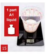
Weigh 1 part of A1 liquid. In this example we use 100 g A1 liquid.
