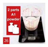
Weigh 2 parts of A1 powder. In this example we used 200 g A1 powder.
