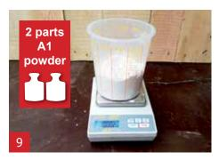
Weigh 2 parts of A1 powder. In this example we used 1000 g A1 powder.
