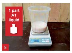
Weigh 1 part of A1 liquid. In this example we used 500 g A1 liquid.
