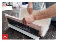
Take the silicone mould carefully from the support mould.
