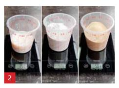
Calibrate the scale and weigh 250 g liquid, 500 g powder and 500 g yellow sand.
