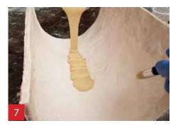
Apply the A1 with a brush in the mould.
