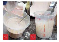
Add the A1 powder slowly to the A1 liquid and stirr with the mixer until you have a smooth mixture 17. Clean the mixer directly after use in water 18.
