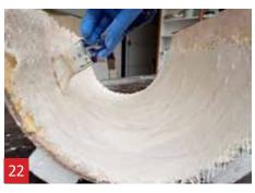
Again apply a thin layer of A1 and smoothen the A1 over the surface.
