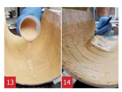
Apply this little amount of A1 on the surface and devide it equally 14. This way you create a smooth finish layer.
