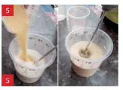
Add sand to the A1 and stir well. Also add 5 g Thix A to the mixture of A1 and sand. (250 g + 500 g = 750 g + 0.5% = 5 g)
