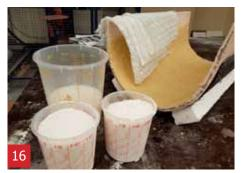
In the meantime weigh 450 g liquid and 900 g powder. Also cut 4 pieces of triaxial fibre same size as the mould you will be using.
