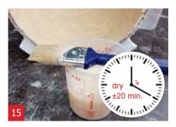
Clean the brush directly after applying the 2nd layer and again let the panel dry for  $\pm$  20 min.
