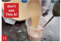
For the 2nd layer of A1 we weigh 125 g liquid, 250 g powder and 250 g yellow sand, and mix them as in step 4 and step 5.
