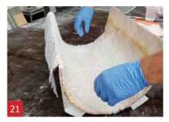
Apply a piece of triaxial fibre with the same size as the object on the surface.
