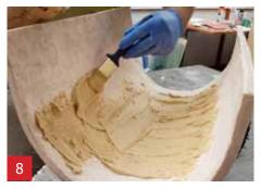
By using Thix A the A1 becomes thicker, like a gelcoat and the A1 won't drop down from the vertical parts.
