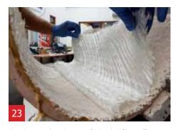
Apply another layer of triaxial fibre. Repeat step 21 and 22 untill you have 4 layers of triaxial fibre. When finished clean the brush with water.
