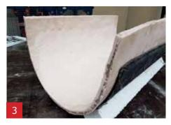
Place the silicone mould into the support mould.
